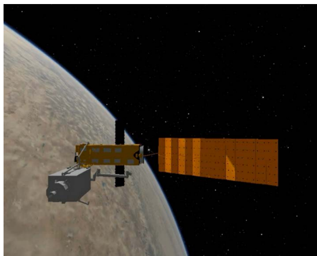
Figure 1: Proximity operation for servicing of ENVISAT satellite (synthetic image with ambient light)
