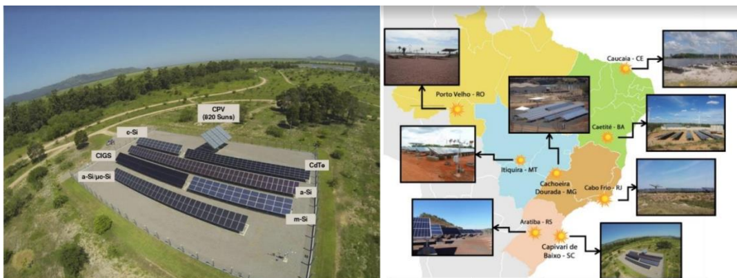
Figure 4. Capivari de Baixo site and the eight identical PV technology test sites located at eight different climatic regions in Brazil.
